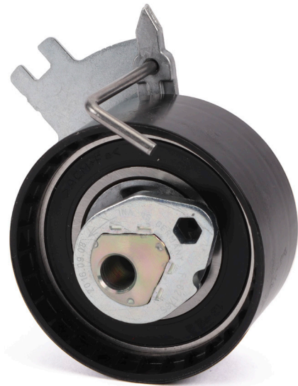
Image 2: Modified tensioner pulley 531 0885 10
